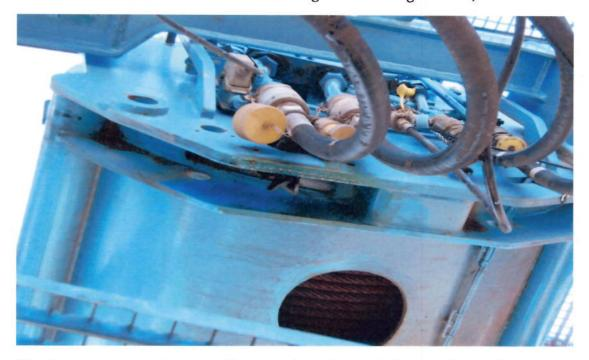
The Upper structure in general looks and works good all controls in cabin where working there was rust on the chrome of both hydraulic A-frame cylinders.
