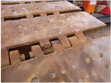
It shows a lot of wear on the pad's where the rollers are rolling on the pads it is to such a degree that the pads don't rotate properly on the pins.
