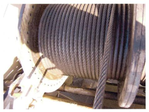
W5 luffer winch is new but doesn't look like it is an original wire and is very sturdy which makes it not easy to assemble luffer (as we have found out in
