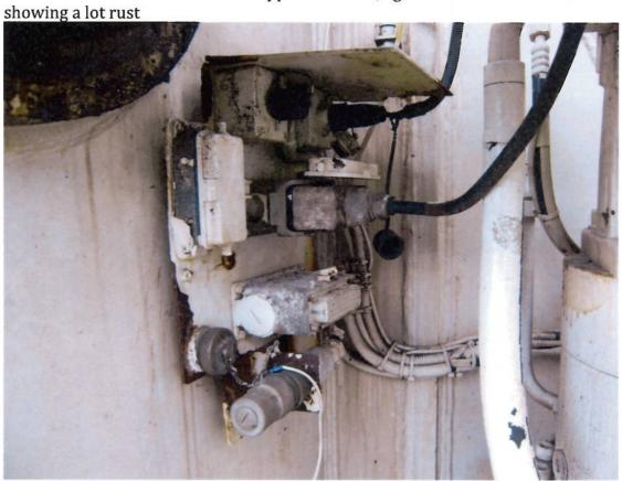
The Luffer looks in good condition there an limit switch broken we could change that whit one of the many heads but still original is broken
