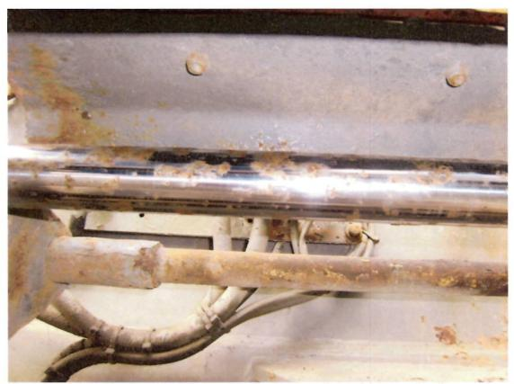
the crome of the hydraulic cilinders to pin the crawlers whit to car body are also very rusty
