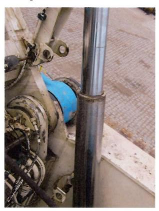
Again rust in many connectors, the engine leaks coolant(minor) and the gear box sweats oil (minor) levels are good. The Hydraulic tank also leaks (minor) and remote control for assembly is not working when open the electric box all screws broke off
