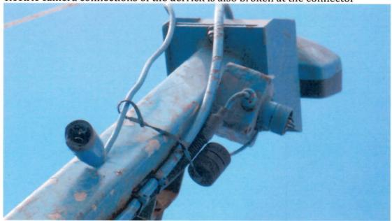
Mainboom electic connections to upper structure, again electric connections are
