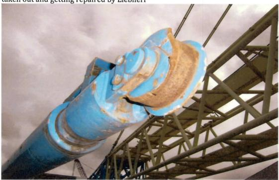
Sheaves of Derrick mast showed a lot of wear of the derrick I changed that whit a sheave from one of the runner attachments. Other sheaves where acceptable
